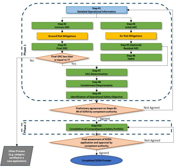
Figure 4 – The SORA process phases
