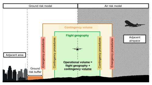
Figure 3 - Graphical Representation of SORA Semantic Model
