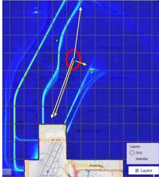
Fig. 2 Las Vegas airport adjacent airspace containment example for near field operations (red circle) with potential flyaway path toward parallel runways (yellow arrow region) or nearby helicopter routes (white arrow region).
