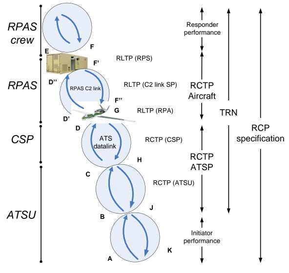
Figure 5 RPAS CPDLC architecture
