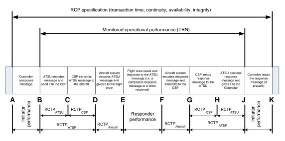
Figure 2 Performance and allocation model from ED-228 / DO-350
