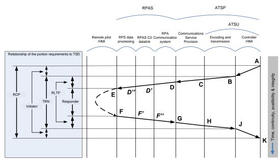
Figure 7 Time sequence diagram for CPDLC in RPAS context
