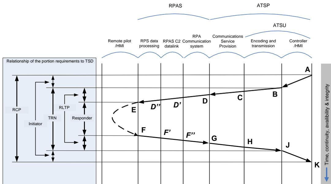
Figure 7 Time sequence diagram for CPDLC in RPAS context
