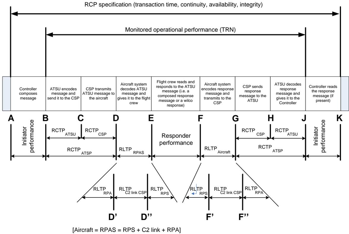
Figure 6 RPAS CPDLC performance and allocation model
