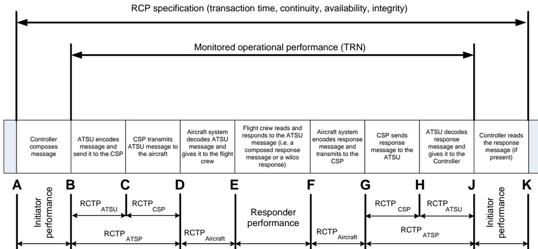
Figure 2 Performance and allocation model from ED-228 / DO-350
