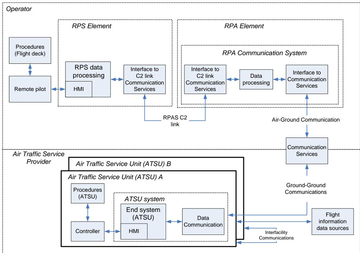
Figure 4 CPDLC application systems and services in the RPAS context (architecture 1)
