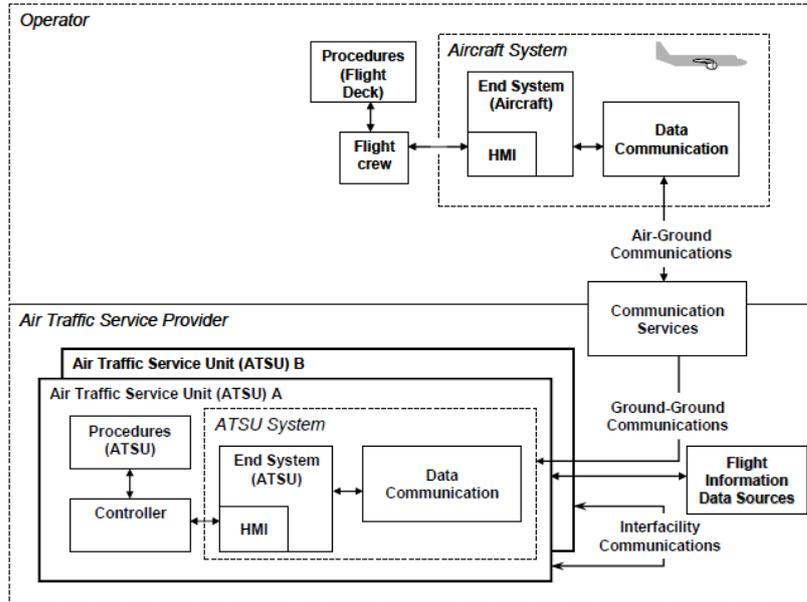
**Figure 1 Overview of the CNS/ATM system (ED-228)**
