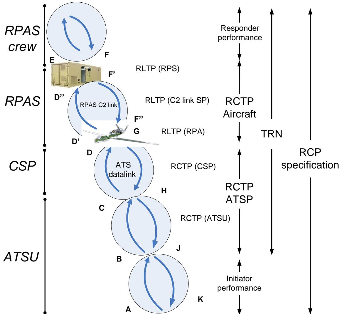
Figure 5 RPAS CPDLC architecture
