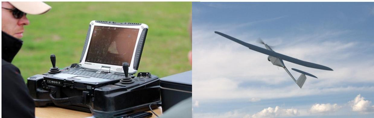
Photo No. 4.5: Station flight management and aircraft FlyEye (a range of about 30 km, altitude: 3000 m flight time 2 h), Source: [www.wb.com.pl](http://www.wb.com.pl)
